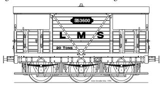
After 1936 the body colour became bauxite and the insignia smaller, probable set out in 3 lines as shown in the drawing below.
